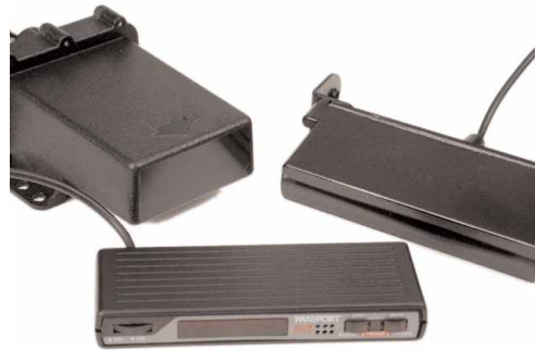
Remote models like Escort Passport SR7 have only a small control/display unit in the cockpit. For the ultimate in concealment, the display can be replaced by single multi-colored status/alert LED built-in to the dash
