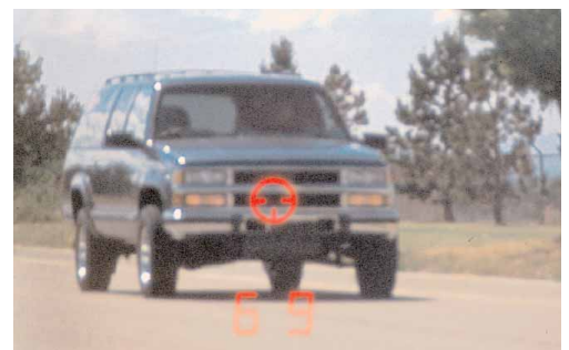
The larger the vehicle, the farther the detector will be from the front plate and the poorer its laser detection.
